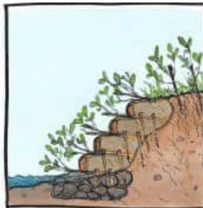
Build encapsulated soil lifts over rock base & toe, plant native woody species.
